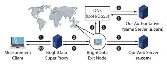
**Figure 1: Our Experimental Setup** —The measurement client, web server, and authoritative name server are under our control. We use proxy service BrightData to reach a large number of clients (exit nodes) located in different countries. Each client sends queries over DNS-over-HTTPS (DoH) and conventional DNS (Do53), and we measure the timing and results.
