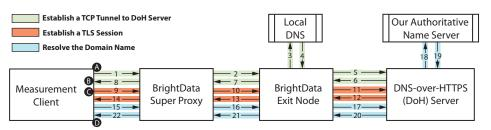
Figure 2: DNS-over-HTTPS (DoH) Request Timeline —Our measurement client sends a DoH request to the BrightData SuperProxy, which forwards the request to an exit node. The exit node then sends a DoH request to an DoH provider (e.g., Cloudflare), which resolves the domain name by contacting our authoritative name server.
