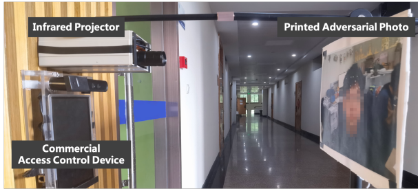
Figure 18. Experimental setup against an commercial access control device. An infrared projector is used to project a structured light scatter pattern onto an adversarial photo of a legitimate user present in front of the target module.
