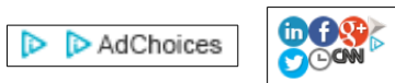
Figure 10: Image Sprites of the AdChoices Logo. Image-sprites are sets of images stored in a single file, and segmented using CSS rules. For example, the left sprite allows to smoothly switch from the icon to the full logo on hover. The right sprite is used by cnn.com to load a variety of logos used on the page in a single request.
