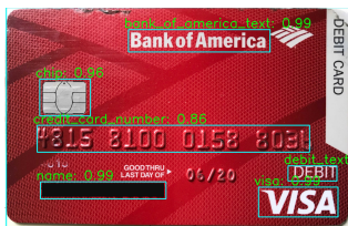
Figure 8: Output of the object detector of the BIN consistency and expectation check. The model correctly identifies, issuing bank, the card network (Visa), card type, chip, name, and card number. These extracted features are correlated with our data of the card BIN to identify any inconsistencies.
