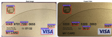
Figure 7: Tampering regions determined by the Faster R-CNN based model [56] on a real image (left), and Fugazi fake (right). Not only does the model fail to detect the tampered regions in the Fugazi fake, it also mistakenly detects untampered regions on both images.
